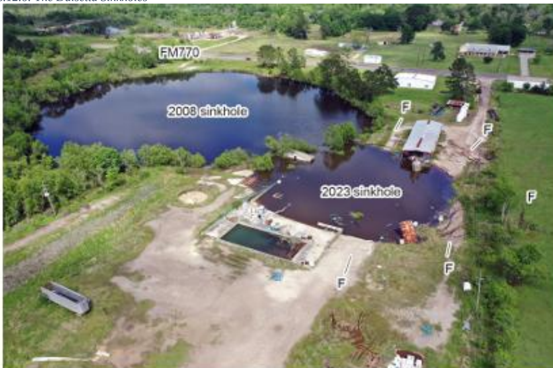
Figure 2. Oblique drone image of the 2008 and 2023 sinkholes, Daisetta, Texas, acquired on April 8, 2023. "F" denotes areas of prominent concentric fissures, scarps, and cracks. View to the east-northeast.
